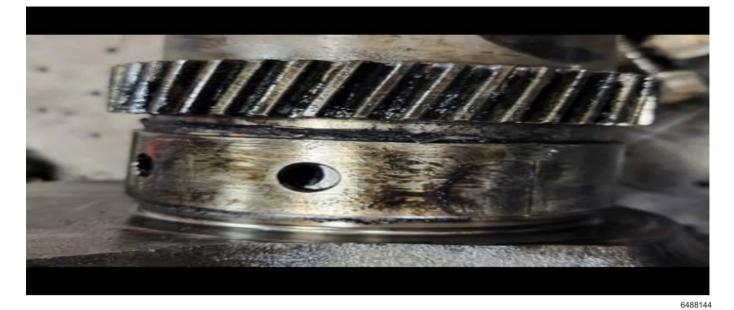
This engine also had oil that was in very poor condition and was full of grit and debris.
