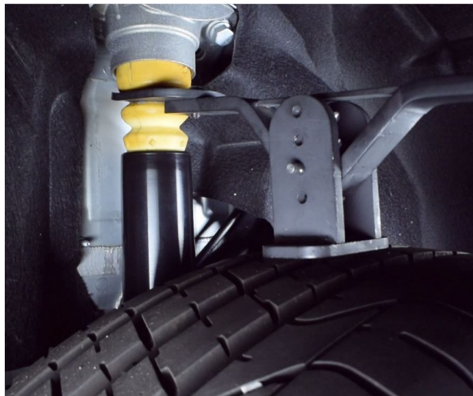
Figure 2. The SET900 tool being used to install a rear bump stop.
