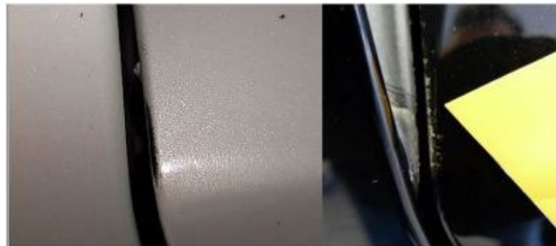
Figure 3. Abrasions in the area of contact.
