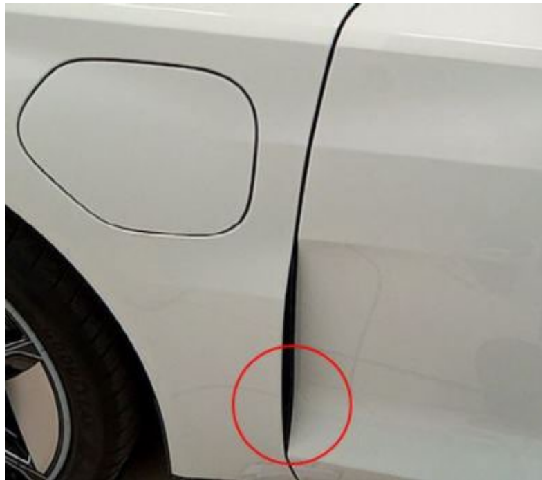
Figure 1. Area of front door affected by the contact.
