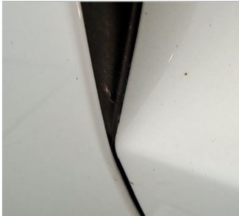
Figure 2. Contact between the front door and the end panel on the front fender when the door is opened.
