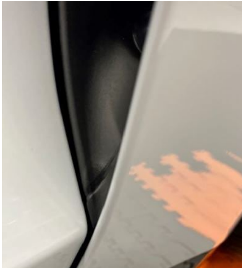
Figure 8. Appropriate clearance restored between the front door and the fender end panel trim.
