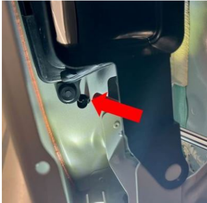
Figure 6. Fully engaged fender end panel trim fastener.
