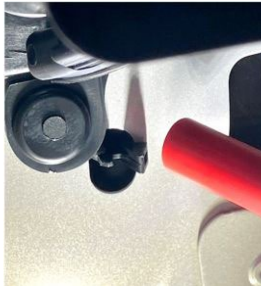
Figure 7. Fender end panel trim fastener properly engaged.
