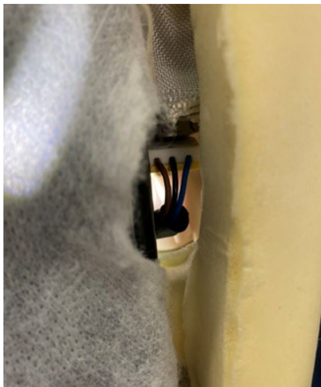
Figure 2. Route new thorax airbag wire harness as close to seat frame as possible.
