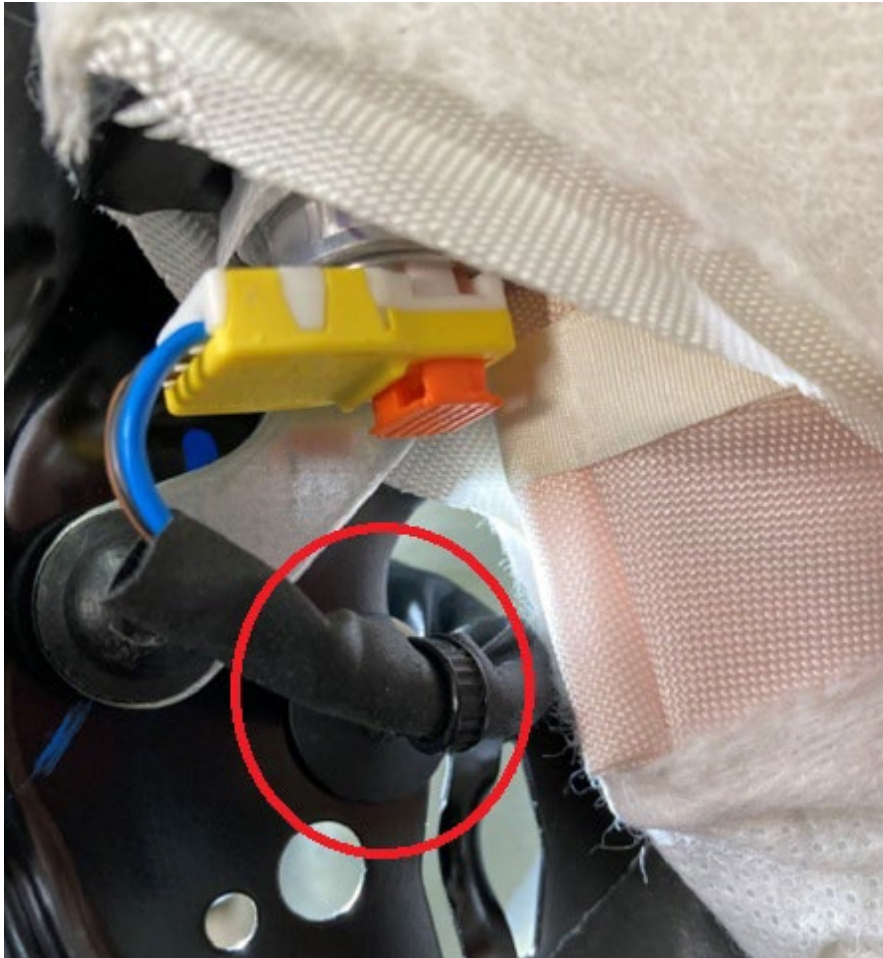
Figure 1. Install additional zip tie/clip when installing new thorax airbag wire harness.
