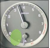
29. Apply **Heavy Throttle Input** from low gear for the <u>engine speed to reach nearly 6,000 RPMs</u>, and allow the ATM to automatically shift to next gear (if equipped w/MT: shift before redline).
