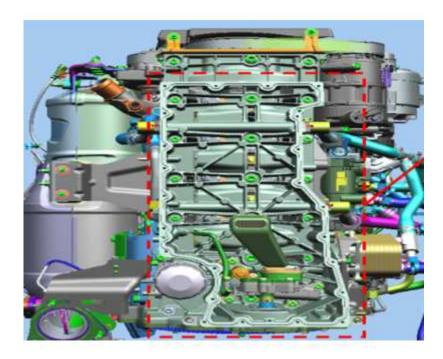
Take one or more pictures of the LCE sealing surface, as shown in the picture above. (NOT REMOVE the RTV from the surface)
