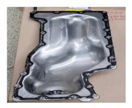
2. Take one or more pictures of the entire sealing surface of the pan dismounted, as shown in the picture above.(NOT REMOVE the RTV from the surface)
