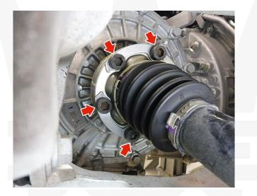
4. Use a Torque Wrench: Follow the workshop manual instructions! Tighten/torque ALL screws following the sequence:
