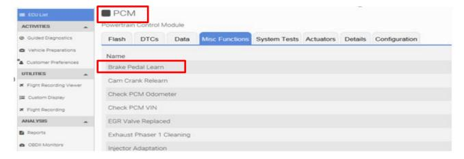
NOTE: If the PCM does not have the above listed "Brake Pedal Learn" option available under the MISC Functions folder, then this SOL publication does not apply, follow the normal diagnostics to resolve.
