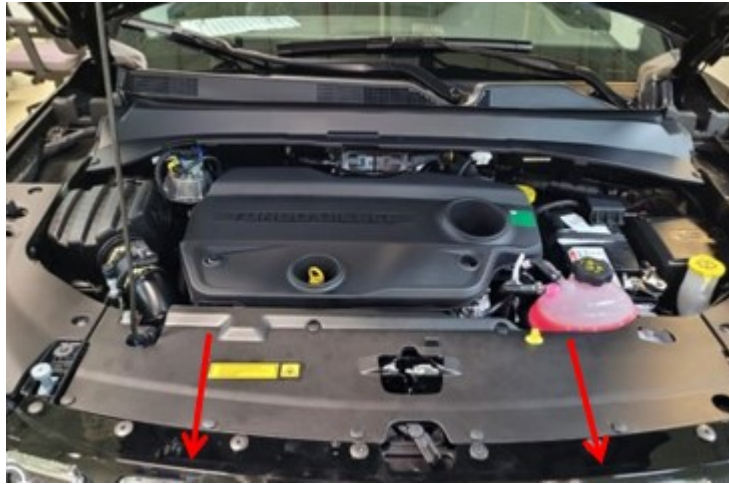
Fig. 1 Radiator Close Out Panel
