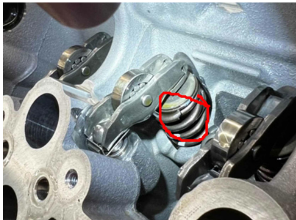
Figure 1 - Broken Valve Spring
