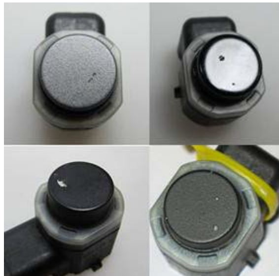
Figure 3. Stone chips causing sensor failure.
