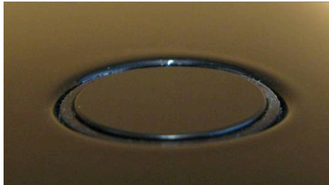
Figure 10. A correctly installed parking aid sensor.
