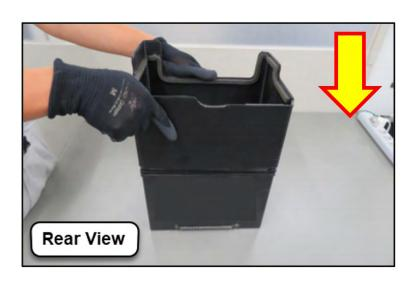
STEP 5: Assemble the new battery holder (p.n. 82184SG000), NEW rear holding rod (p.n. 82161SJ000), and the ORIGINAL front holding rod as shown below. The original rod nut can be transferred to the new rear holding rod.
