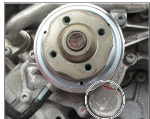
Traces of coolant on coolant pump
