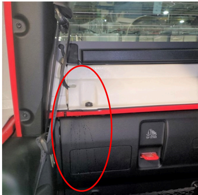
Fig. 1 Water Leak At Backlite
