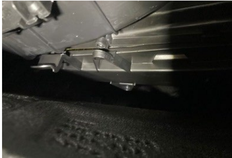
Figure 1. Cover for the dust and pollen filter not fully engaged.
