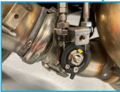
Fig. 2 – Exhaust flap control (Heat shield removed)
