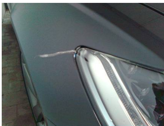
Figure 1. Car wash bristle stuck in body gap.
