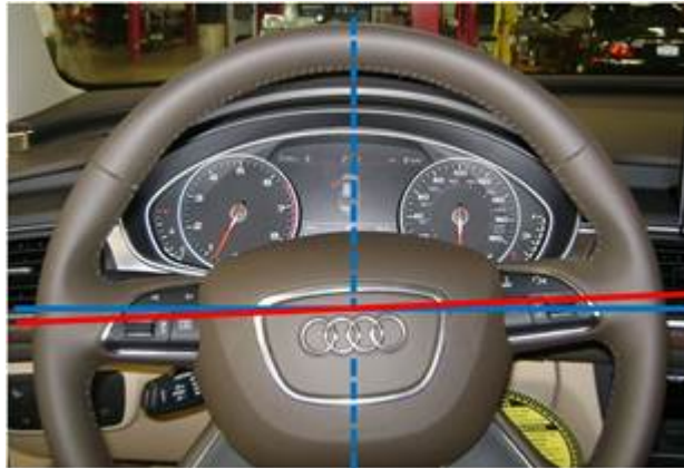
Figure 1. Steering wheel not leveled (off-center)
