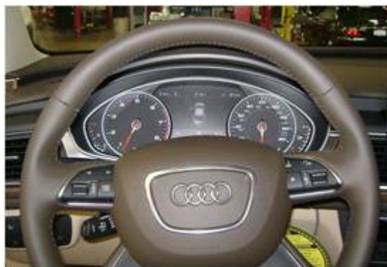
Figure 3. Example of a steering wheel not leveled (off-center) condition.
