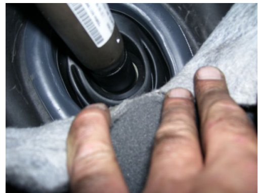
Figure 2. The sealing sleeve on the bulkhead.
