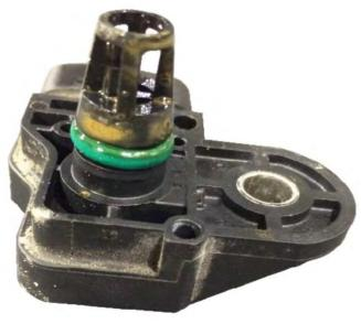
**Important:** Due to the sensitivity of the sensor, **Do Not** use any chemical cleaners including water and **Do Not** use compressed air to remove contaminates.
