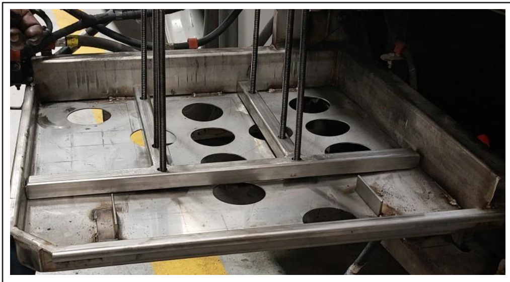
Figure 5 - Installation of Brace to Tray Bottom
