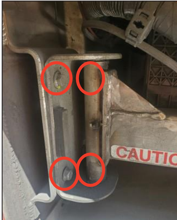
Figure 2 - Location of Battery Tray Hinge Bolts
