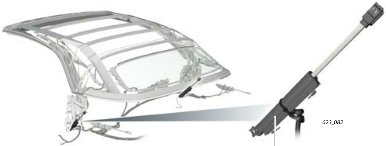
Hydraulic cylinder of main bearing , (left hand side)
