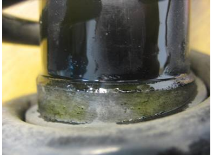
Figure 1. A leaking shock absorber.
