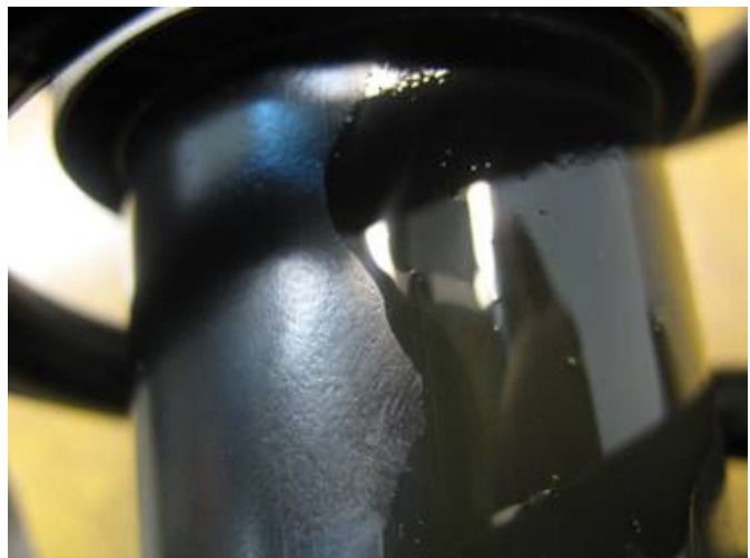
Figure 2. A leaking shock absorber.
