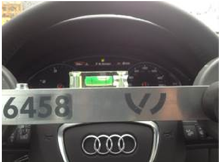
Figure 3. Example of a steering wheel that is not level.
