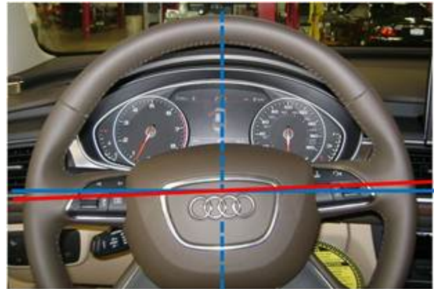
Figure 1. Steering wheel not leveled (off-center)
