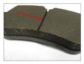
Figure 3. Clean brake pad groove.
