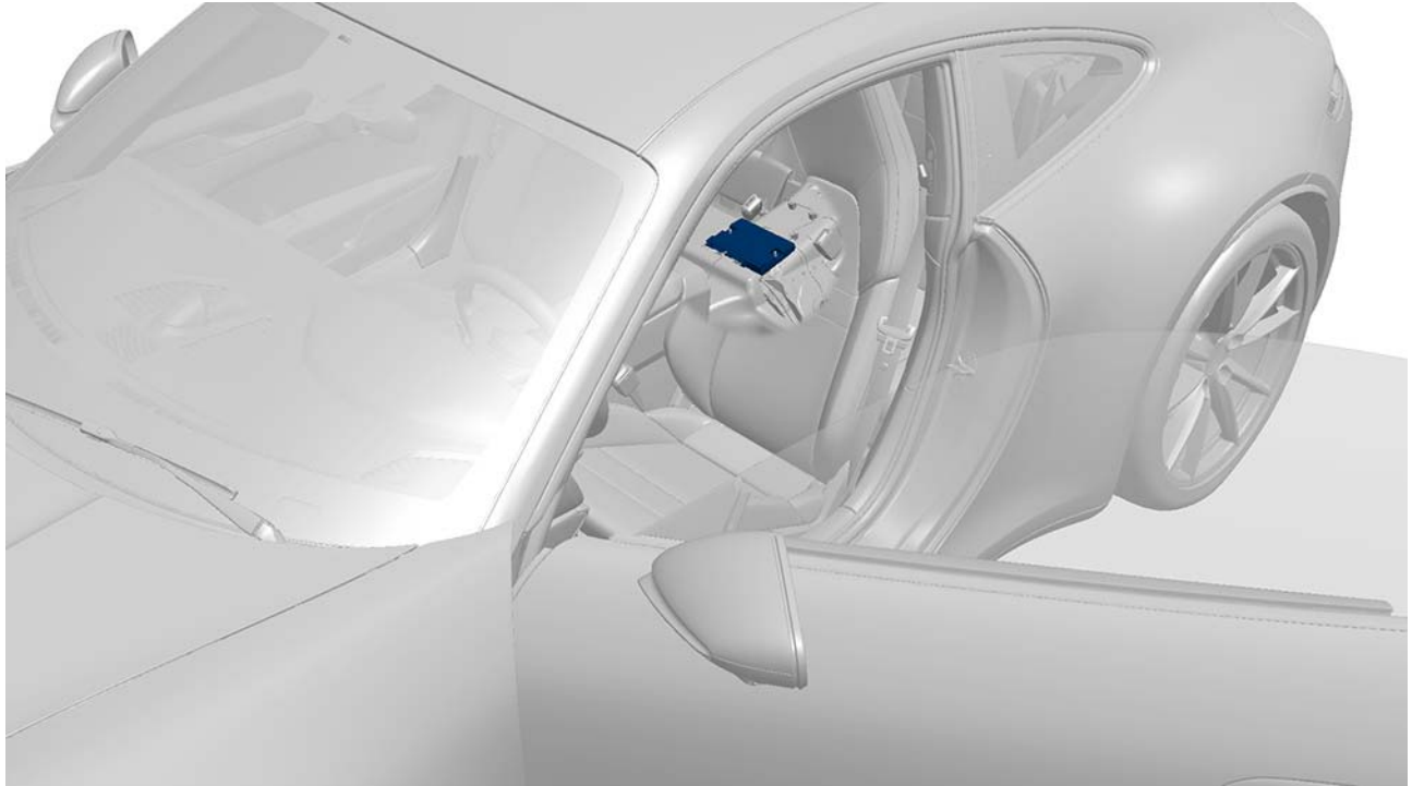
Installation position of gateway control unit
