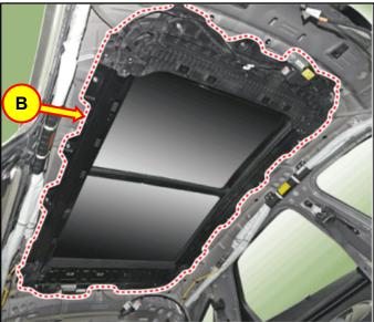
4. Place a shim on each section of the panoramic sunroof to prevent excessive movement during adjustment.
