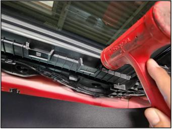
6. Measure all 4 locations of the sunroof again to ensure they are within the specified range (12 – 14 mm). Readjust if needed.
