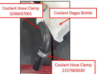
**7**. Install the new coolant degas bottle using the four fasteners previously removed. Tightened to the specified torque.
