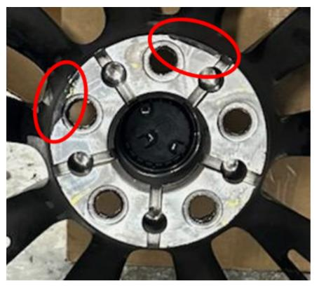
Above Image shows paint on the hub surface of the wheel, this paint may also get transferred to the hub bearing surface.
