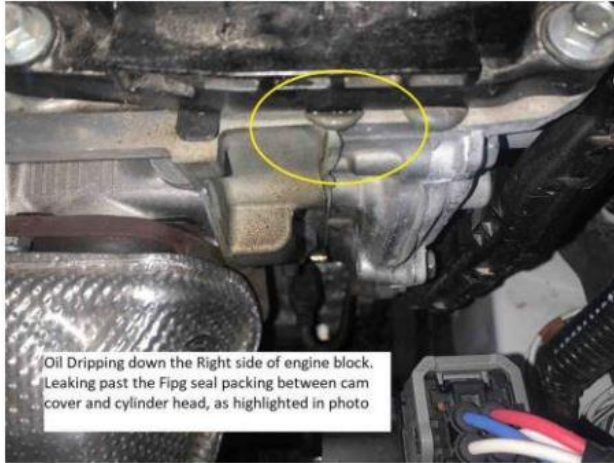
Figure 2. Images of head/valve cover gasket leaks.
