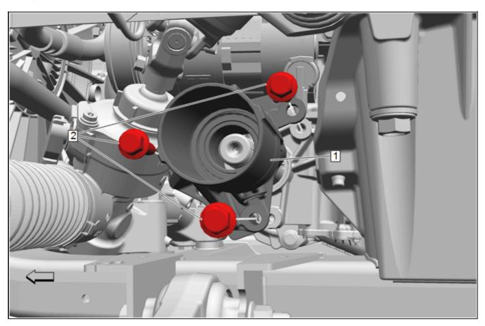
1. Remove the front wheel drive intermediate shaft housing (1). Refer to *Front Wheel Drive Intermediate Shaft Housing Replacement* in SI.
