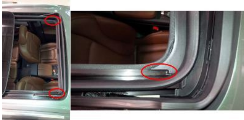
Figure 5. Areas of the sunroof frame to be isolated with webbing adhesive tape.
