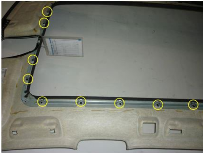
Figure 1. Location of the headliner to sunroof frame clips.
