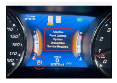
DTCs in ECU: in AFLS ECU are present the following DTC:
