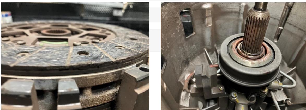
Figure 9: checks of the wear of the friction material of the clutch plate (left) and of the status of the clutch thrust bearing (right).
