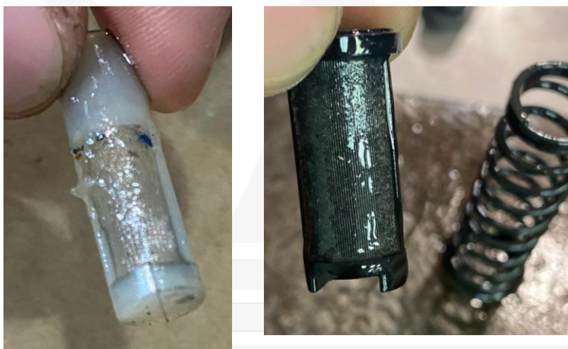
Figure 8: filters of the F1 hydraulic actuation circuit. In this case, they were found to be dirtied by metal shavings.
