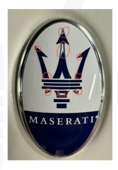
The result of the analysis confirmed not only a lack of the coating material but also a lack of paint caused by a polishing of the component done using an orbital polishing machine.
