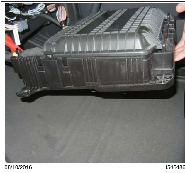
Fig. 1, Lowering the VPDM to the Cab Floor
