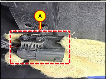
2. Apply the supplied vinyl sheet (B) to the front bumper main wiring connector to overlap the wiring creases and wind the connector wiring so that it cannot be seen.
