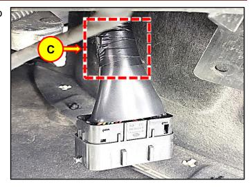
4. Wrap the PVC tape between the connector and the wiring so that the wiring in the area (D) is invisible.
