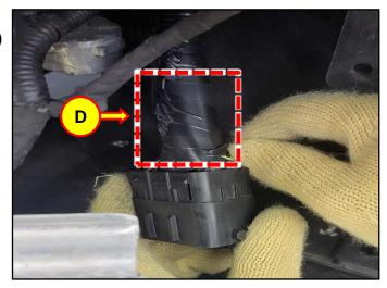
5. Install the connector (E) on the connector mounting area.
