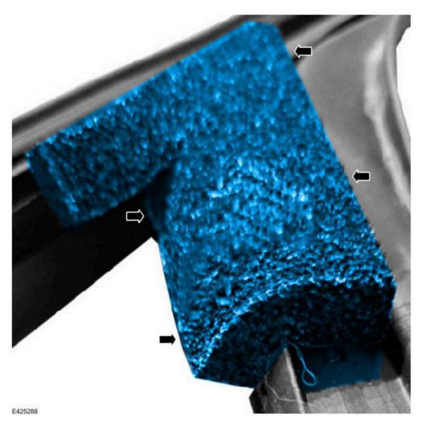
16. Moving to the exterior of the glass top run, take the end of the foam extension and pull, seating the foam toward the header/A-pillar corner.
