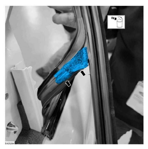
12. Clean the surface to remove any residual foam.
