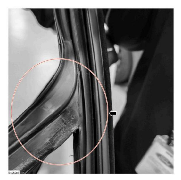
13. CAUTION: Be careful to not tear the rubber of the glass top run when fitting/tucking the foam underneath.
