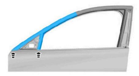
5. Insert the front of the foam first making sure is seated under the window run/sheet metal and the foam shape properly fits the curves of the door (see Parts Required).
