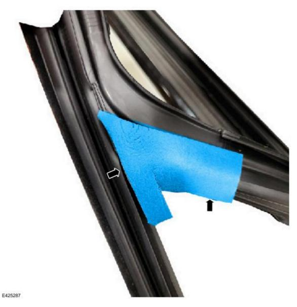
15. Fold and pressurize the lower area of the foam over the back of the A-pillar channel, leaving the upper extension unadhered.
