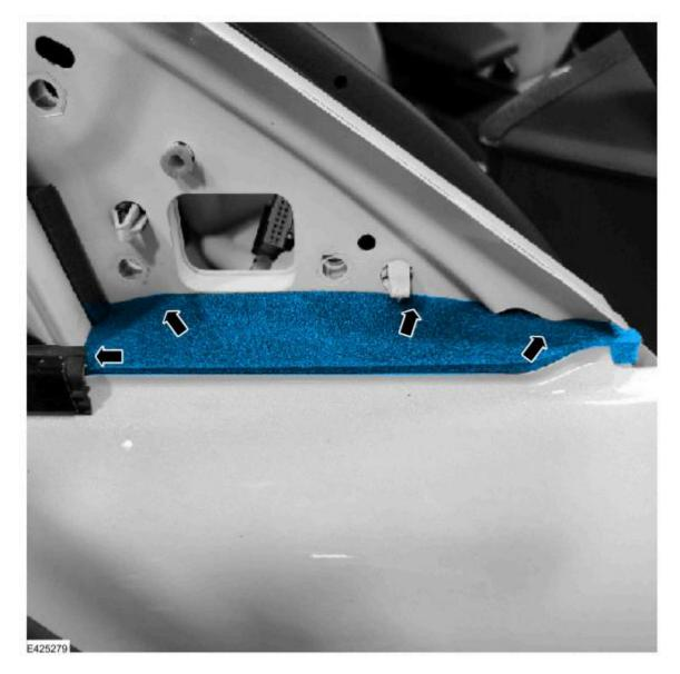
6. Evenly tuck all edges of the foam into the door making sure that the rear sections sit flush against the window run frame with no gaps.
