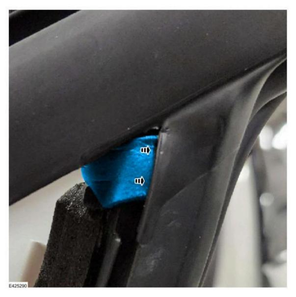
18. Reinstall the front door glass top run in the door frame and the run channel.
