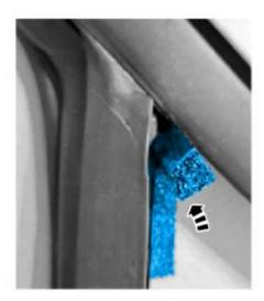
17. Tuck the end of the foam extension high up under the lip of the glass top run following the upward angle of the run.
