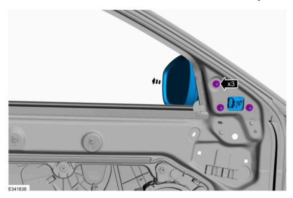
3. If the exterior mirror foam gasket/seal remains on the door, remove and refit the mirror foam gasket/seal back onto the mirror before reassembly.
