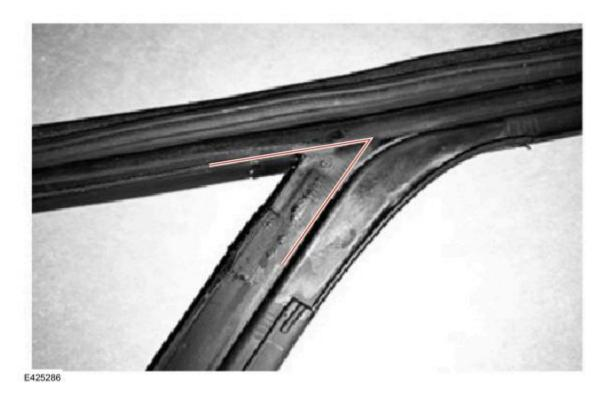
14. Apply pressure to adhere the foam to the inner surface of the glass top run.
