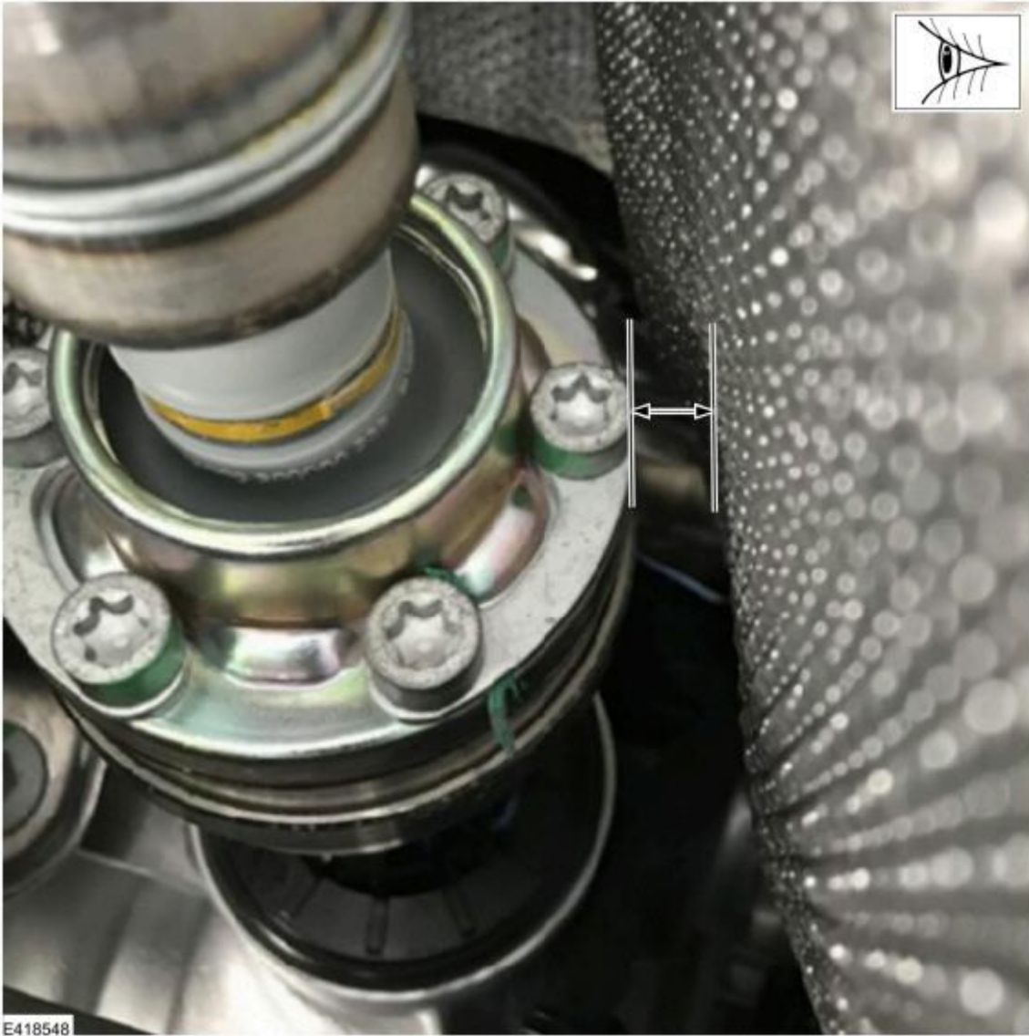
Figure 2 - Example of rubbing marks on the driveshaft fasteners
