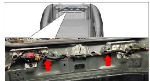
Constriction for main wire harness
