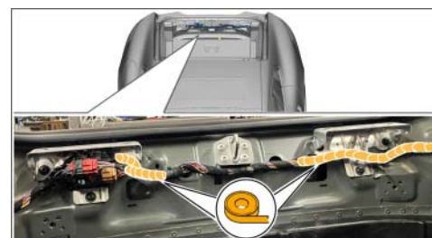
Wrapping main wire harness in luggage compartment
