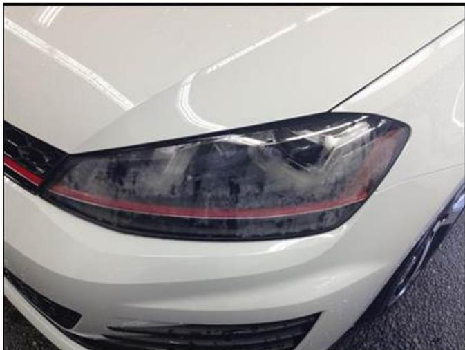
Exterior light assemblies (headlights, taillights, fog lights, turn signals) are vented and may collect moisture on their inner surfaces, depending on humidity and climatic conditions. The unfavorable condensation built up (Figure 1) visible to the customer is more common with modern exterior lights because of clear glass optics, however this condition will not have an impact on the functionality or durability of the component.
