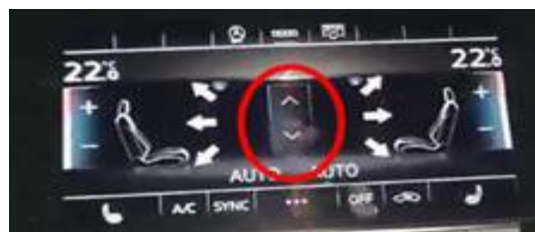
Figure 1. Normal HVAC control panel appearance.
