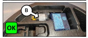
If sealant <u>has</u> leaked from the TMK sealant can (NG), replace the sealant can (B), <u>take one (1) clear KVID photo</u> and proceed to 'Repair Procedure' step 5.
