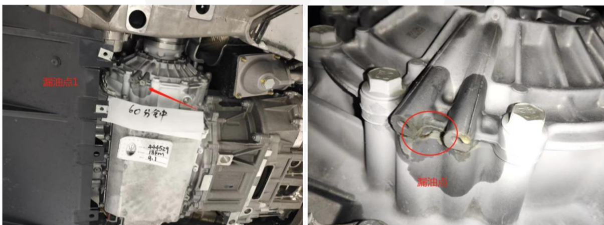
Example of oil leak around the differential area
