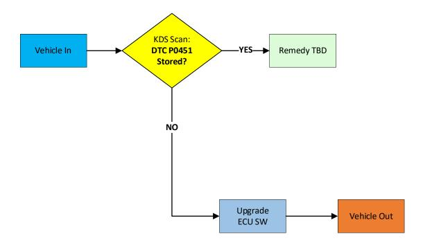
Path 1: Vehicle IN → Related DTC stored (NO) → Upgrade ECU SW → Vehicle OUT
