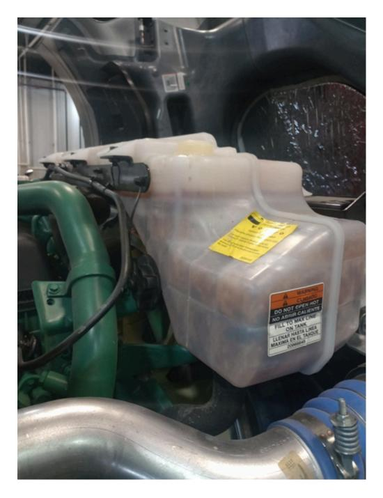
If the truck is unacceptable to be driven with the contamination (dark color, large deposits of debris), please start an e-service case (directed to the Reliability Group) to document the issue. Flush the coolant (per IMPACT 2609-11-03-01) and install a new coolant filter, over flow tank, and fill with new coolant.
