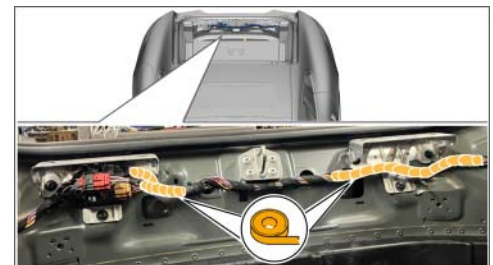
Wrapping main wire harness in luggage compartment
