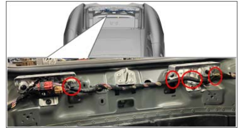
Checking main wire harness in luggage compartment
