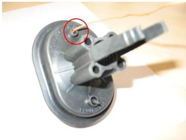
Figure 6. Access hole in grommet to be sealed with Butyl sealant.
