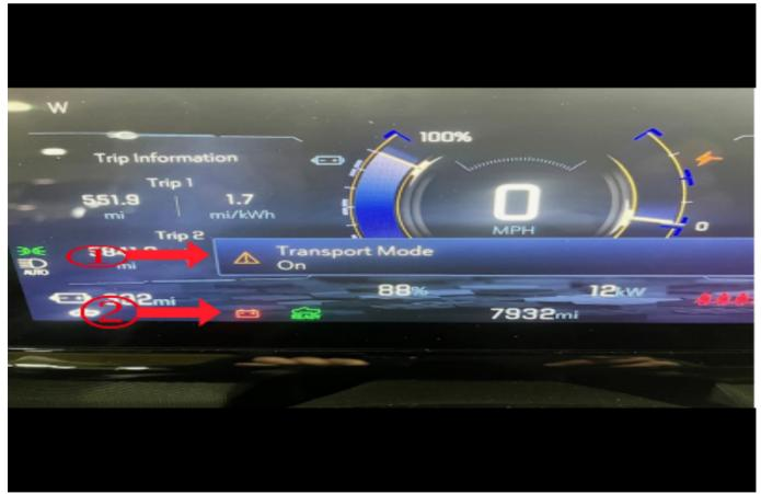
6. When Transport Mode is enabled, a message will display on the DIC (1), and the Battery Warning light (2), as shown in the photo above will flash.
