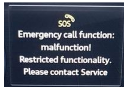
Figure 1. Emergency call malfunction warning.
